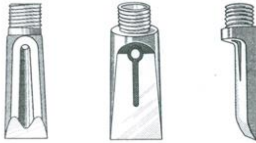
Fig. 12.5. Types of jetting drill bits. (Source: Todd, 1980)
